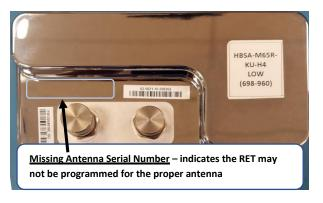
Any RET not labeled with the antenna serial number must be assumed to be a raw bulk spare and the same warnings noted above will apply.
